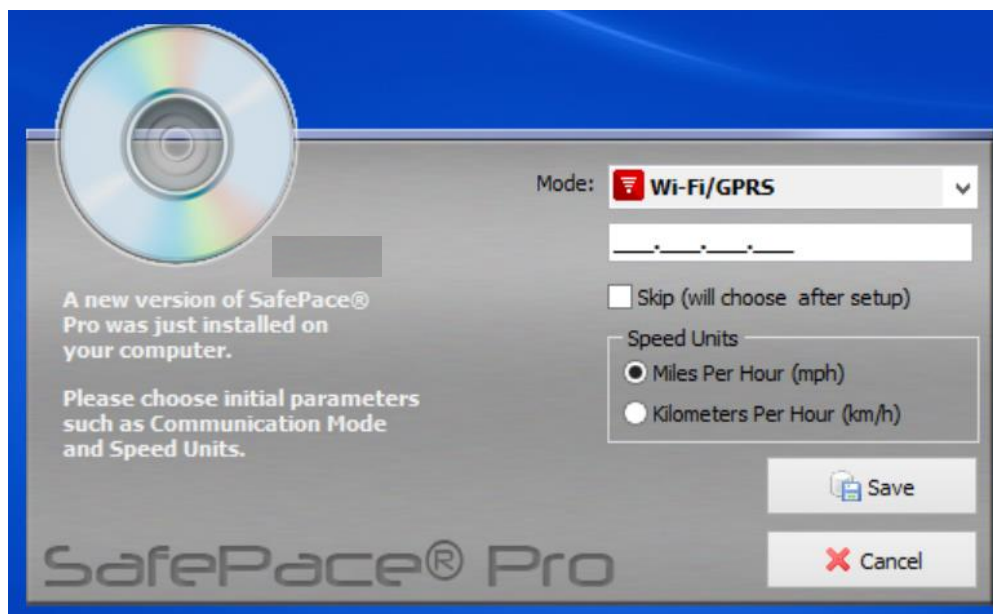
Figure 22 – Initial settings window – GPRS mode – enter static IP address for SIM card module
