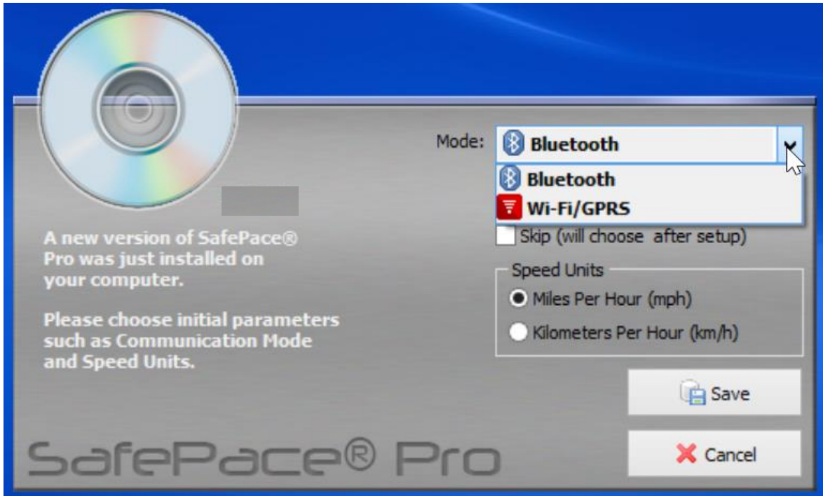
Figure 17 – Initial settings window – set communication mode and speed units
